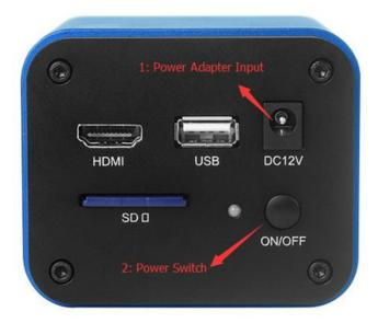
As seen in the above picture, to power on the camera, please plug the power adapter into the DC12V port first. At this time, the LED on the back panel will be turned on and shown as red. To put the camera into a working state, please push the On/Off button once. Then the LED will switch the color from red to blue. The blue LED indicates that the camera is working now.
