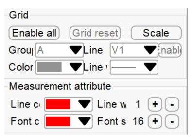
Click the "All" button to turn on 8 horizontal and vertical scale lines. User can turn on or off any grid line base on your need. User can also set up the color and thickness of each line. Under the "Group" option, it can save 8groups of grid lines, which is convenient to open the set grid lines quickly when testing the product.
